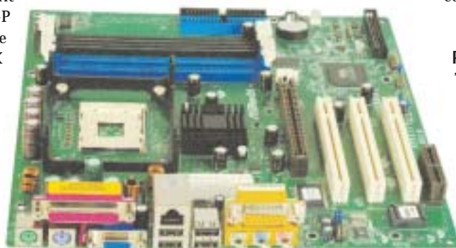
The ASRock M266A motherboard has a micro ATX form factor and hence comes with a cramped layout
